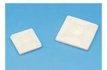
Material: UL approved Nylon 66, 94V-2 (Backed with adhesive tape) Self-Adhesive TIE Mounts is designed to support light weight wire bundles when properly applied on any clean, smooth, grease-free surface. For heavy support. mounting hole is provided for screws. To apply, simply peel off backing paper and apply mount to surface. After that, cable ties can be inserted to secure wire bundles. Black color available
