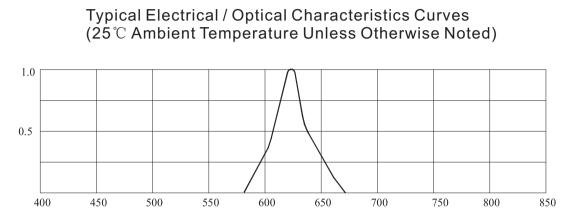
$Wavelength \ \lambda \ (nm) \\ Fig. 1 \ Relative \ Intensity \ vs \ . \ Wavelength \$
