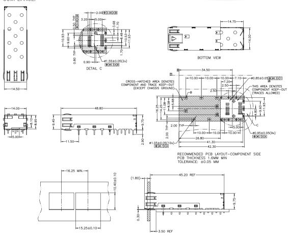
RECOMMENDED BEZEL CUT-OUT CENTER DETAIL BEZEL THICKNESS 0.8 $\sim$ 2.6MM
