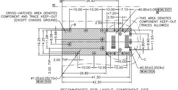
RECOMMENDED PCB LAYOUT—COMPONENT SIDE PCB THICKNESS 1.6MM MIN TOLERANCE:  $\pm 0.05\,$  MM
