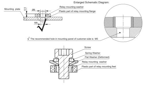
When use M5 screw, the thickness and strength of the washer needs to be guaranteed or it may deform and burst the cover.
