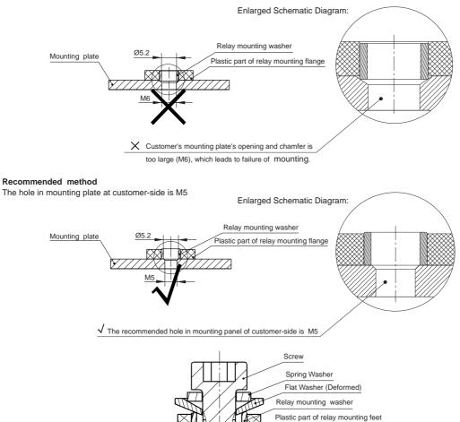
When use M5 screw, the thickness and strength of the washer needs to be guaranteed or it may deform and burst the cover.
