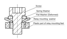
When use M5 screw, the thickness and strength of the washer needs to be guaranteed or it may deform and burst the cover.
