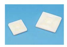
Material: UL approved Nylon 66, 94V-2 (Backed with adhesive tape) Self-Adhesive TIE Mounts is designed to support light weight wire bundles when properly applied on any clean, smooth, grease-free surface. For heavy support. mounting hole is provided for screws. To apply, simply peel off backing paper and apply mount to surface. After that, cable ties can be inserted to secure wire bundles. Black color available
